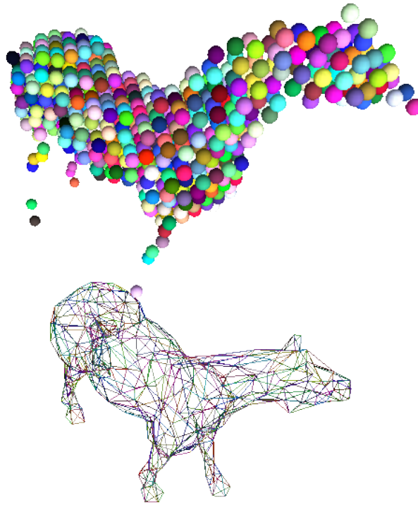
Fig. 3.3: Imported GTS surface (horse) used as packing predicate (top) and surface constructed from facets (bottom). See http://www.youtube.com/watch?v=PZVruIIUX1A for movie of this simulation.
