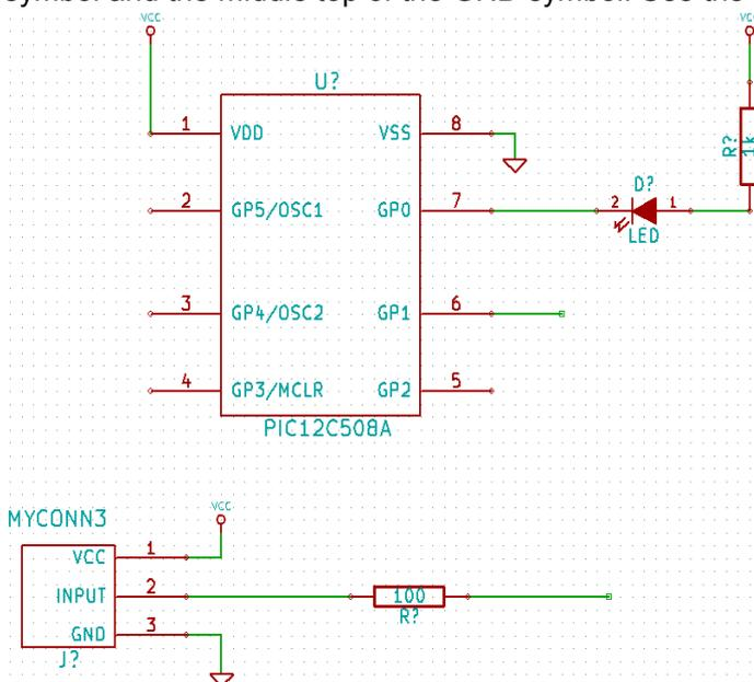
32. We will now consider an alternative way of making a connection using labels. Pick a net labelling tool by clicking on the 'Place net name' icon
