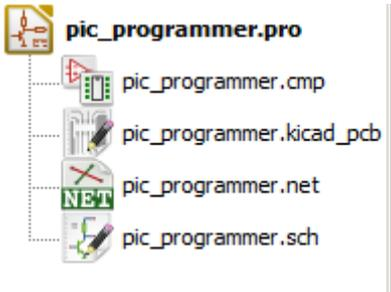
Double-clicking on the Eeschema icons runs the schematic editor which in this case will open the file pic\_programmer.sch.
