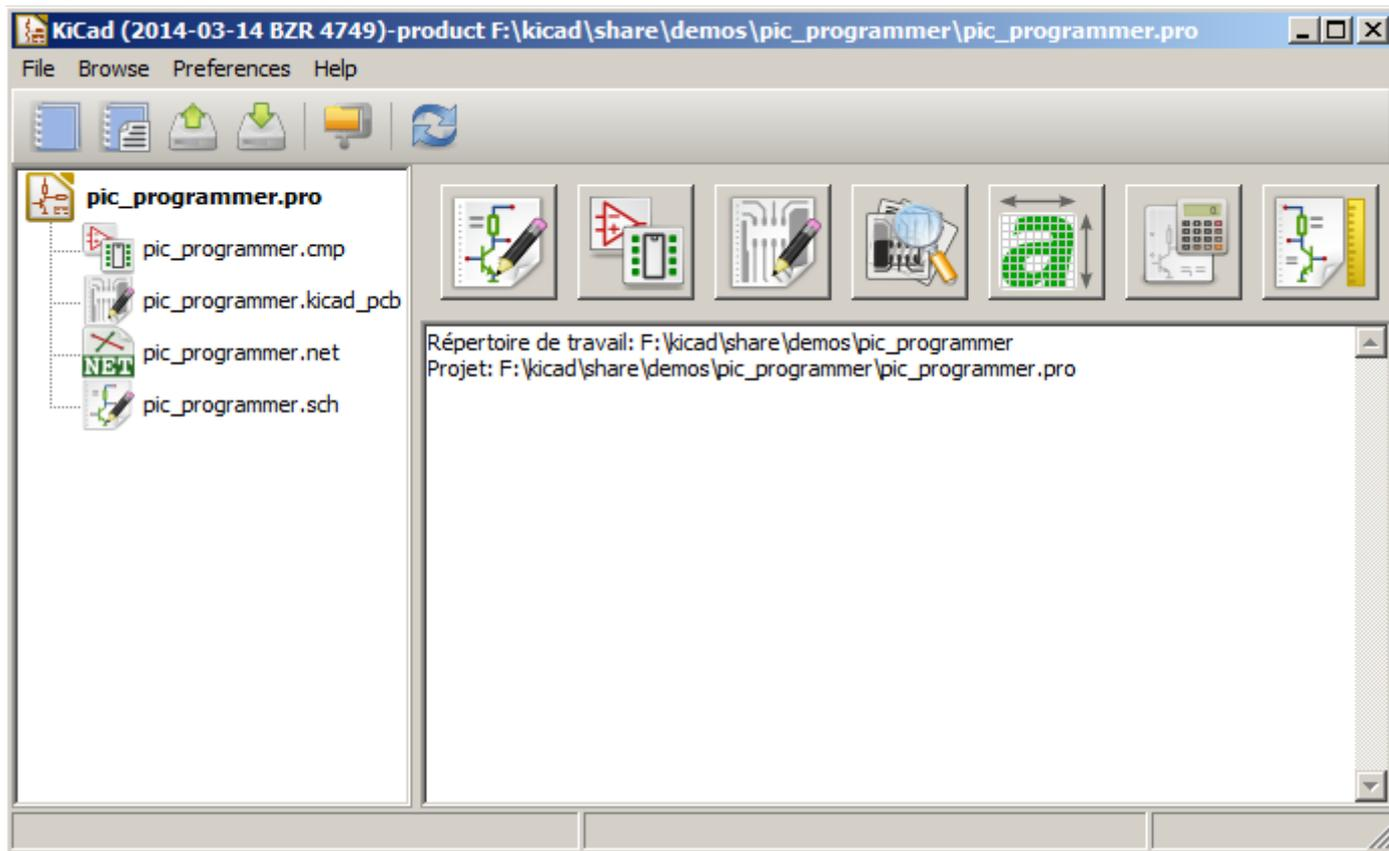
The main KiCad window is composed of a project tree view, a launch pane containing buttons used to run the various software tools, and a message window. The menu and the toolbar can be used to create, read and save project files.
