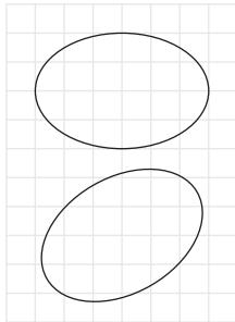
`\Oval` draws an oval. The first pair of values is the center of the oval. The next pair forms the half-height and the half-width. The last argument is a (counterclockwise) rotation angle. The interior is transparent, so that it does not erase previously drawn material.
