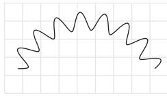
In this command we have one coordinate: the center of the circle. Then follow the radius of the circle, the start angle and the finishing angle. The arc will be drawn counterclockwise. The final two parameters are the amplitude of the wiggles and the number of wiggles. Like the other commands in this section, this command can take optional arguments, Sec. 5.5.
