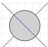
`\GCirc` draws a circle with the center at the specified coordinate (first two arguments) and the specified radius (third argument). Previously written contents are overwritten and made gray according to the grayscale specified by the fourth argument (0=black, 1=white).
